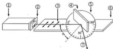
Fig. 9. Experimental setup of measuring Brewster’s angle
