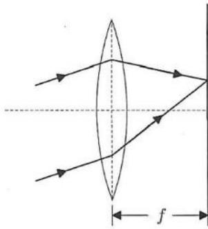
Fig. 1. The focal plane of a convex lens
