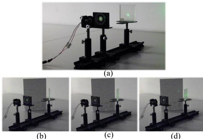
Fig. 10. Experimental setup of measuring Brewster's angle.
