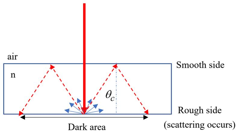
Fig. 4. Total internal reflection (TIR) between air and acrylic plate.
