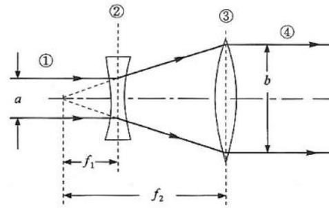
Fig. 2. Beam expander. ①incident light ②concave lens ③convex lens ④outgoing light
