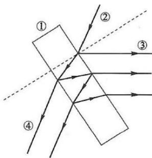
Fig. 3. Expansion of the beam size by a glass plate ①glass plate ②incident beam ③reflected beams ④transmitted beams
