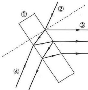
Fig. 3. Expansion of the beam size by a glass plate ①glass plate ②incident beam ③reflected beams ④transmitted beams
