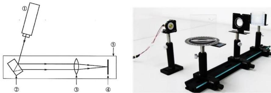
Fig. 5. Experimental setup of measuring the focal length of a thin convex lens.
