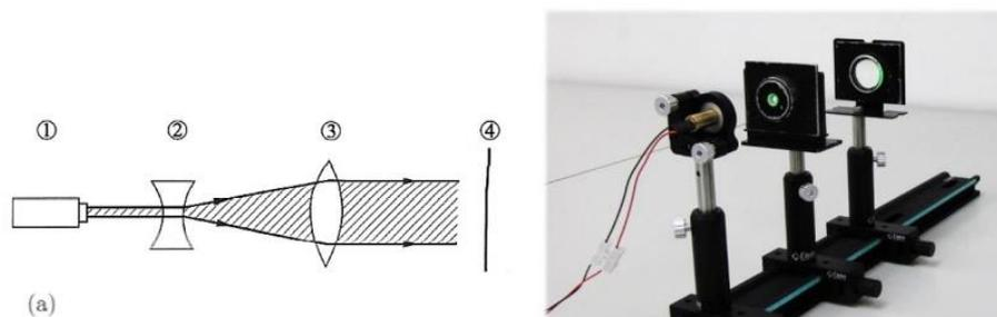
Fig. 6. Experimental setup of measuring the focal length of a thin concave lens.
